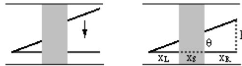
Figure 8: Example of seam width calibration. After the user fits the line on the right side, the seam width x_S can be computed as x_S = (h / \tan \theta) - (x_L + x_R) .
