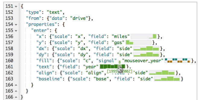
Figure 1. Code augmentations visualize the runtime state of program variables in a Vega [32] specification. A histogram shows the distribution of variables containing set data. Interacting with the year histogram filters all other histograms to only show the data values where the year is between 1995 and 2002 (hand cursor shown here for clarity; in a real implementation the cursor is hidden mid-interaction to aid chart reading). For mouseover_year , a tick visualization depicts value changes.
